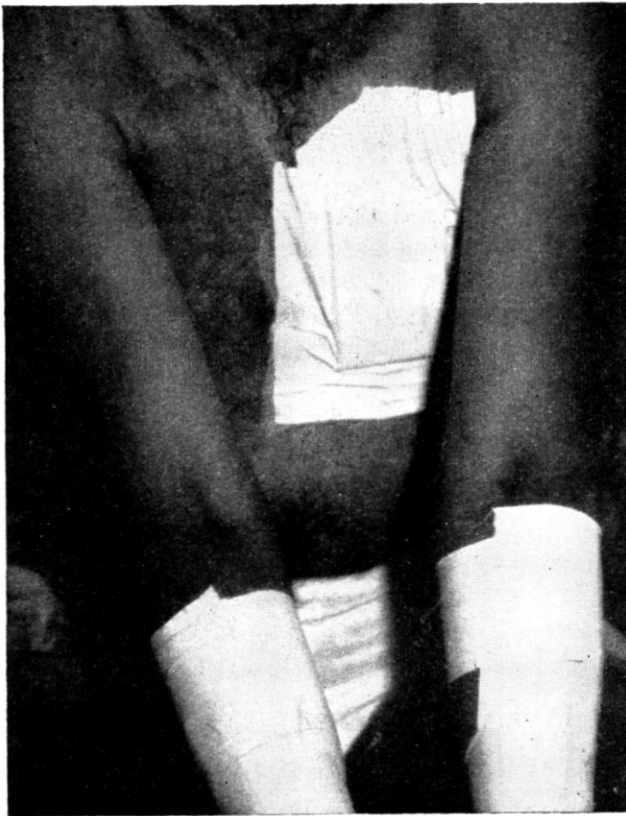
FIG. 2. Picture of subject before flight showing the position of track plates located on chest and arms (print reversed).
